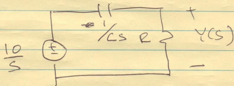
$$\begin{aligned} V(s) &= \frac{R}{\frac{1}{Cs} + R} \frac{10}{s} \\ &= \frac{RCS}{1 + RCS} \frac{10}{s} = \frac{10}{s + \frac{1}{RC}} \end{aligned}$$
